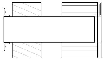
adhesive gently against the wall, compressing the adhesive somewhat. Then pull the tube into the room leaving the finisher in place. Ensure that the finisher does not fall.
