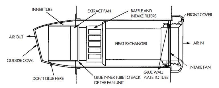
**k)** Now fit the wall plate to the wall. The wall plate is marked top on the front face. If the sleeve on the rear wall plate does not fit into the drilled hole, carefully open up the hole in the plasterwork until the wall plate will fit flush against the wall and is central in the drilled hole. (Use the remnant piece of large diameter tube as a template to ensure it is central).
