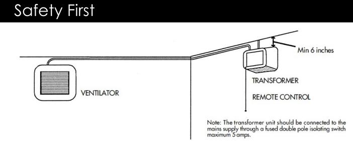
The Heat Recovery Ventilator is a "SELV" (Safety Extra Low Voltage) ventilator that operates at 12 volts AC. Under no circumstances must this be connected directly to the mains supply. Damage so caused is not covered by the warranty. The isolating transformer / humidity sensor supplied must provide the low voltage used by the ventilator. A typical layout of installation is shown above.
