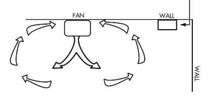
**m)** The Transformer / Humidity sensor unit may be mounted on the wall or ceiling.
