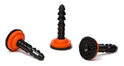
Place the membrane in position as level as you can judge by eye. Using a 10mm drill bit, drill through the centre of a stud near the top and edge to a depth greater than the fixing. The fixing is then hammered into the pre-drilled hole until the seal compresses tightly into the stud. The rubber washer re-seals the hole. Level the membrane using the spirit level or laser level if used, and fix another plug about 2m along at the top of the sheet. The membrane will now be hanging level to the wall.
