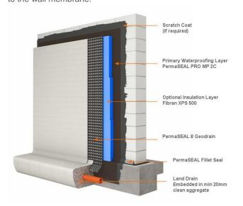
PermaSEAL 8 Geodrain is supplied in 2m wide rolls. If the foundation wall is less than 2m in height it is possible to fix PermaSEAL Geodrain horizontally with no laps. For walls over 2m fix PermaSEAL 8 Geodrain in vertical sheets with the Geotextile fabric layer facing the backfill and the black drainage layer against the wall being waterproofed.
