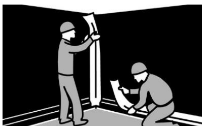
(Fig. 4) Before applying PermaSEAL Self-Adhesive Tanking Membrane to larger surfaces, cover all outside corners, edges, valleys, etc. with cuttings and reinforcement strips so that all risky areas are covered by two layers of the membrane when the installation process is complete. Strips should be approx. 200 - 300 mm wide. Remove the paper from one side and glue on the PermaSEAL Self-Adhesive Tanking Membrane strip. Next, mould the strip more closely to the surface, pull off the other half of the backing paper and seal the sheet.
