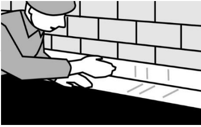
(Fig. 22) Cover the transition from the floor to the masonry with a strip no less than 300 mm wide.
