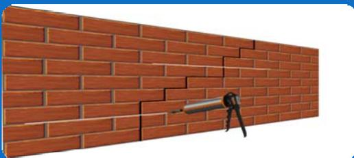
Apply a second bead of grout into the slot making sure that the bar is completely covered and with the trowel provided force the grout into the slot until it is approximately 10mm from the surface and ensuring that the bar and grout are firmly packed.
