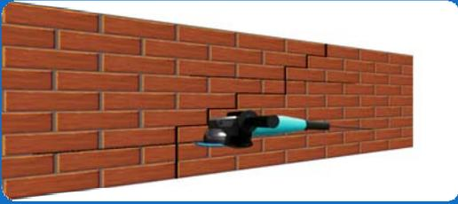
Cut a slot in the mortar bed just over 500mm either side of the vertical crack and to the correct depth, dependent on the wall thickness (see below). Remove the mortar including all loose material and then flush the joint with water. Normally vertical spacing is every 4 - 6 brick courses but check with a structural engineer if in doubt.
