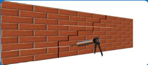
Mix the grout thoroughly using the paddle mixer provided and load into the gun. Pump the grout to the back of the slot in a continuous even bead to approximately two thirds of the slot depth.
