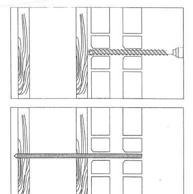
1. Drill a 14mm hole through both brick outer and inner leaf.
