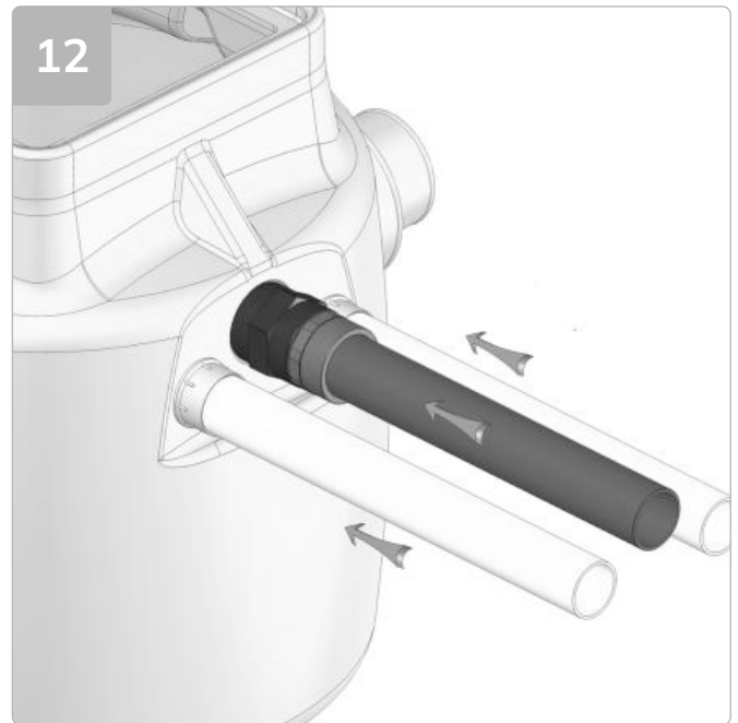
Push discharge, cable duct and vent pipe into their respective male iron, twisting the pipe as it is pushed into the male iron to remove any trapped air.
