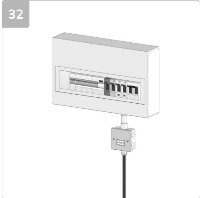
Isolate mains supply and connect the pump and high level alarm according to the wiring diagram overleaf.
