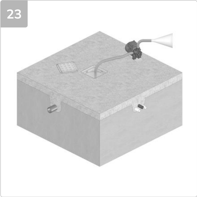
Pump out water from chamber.
