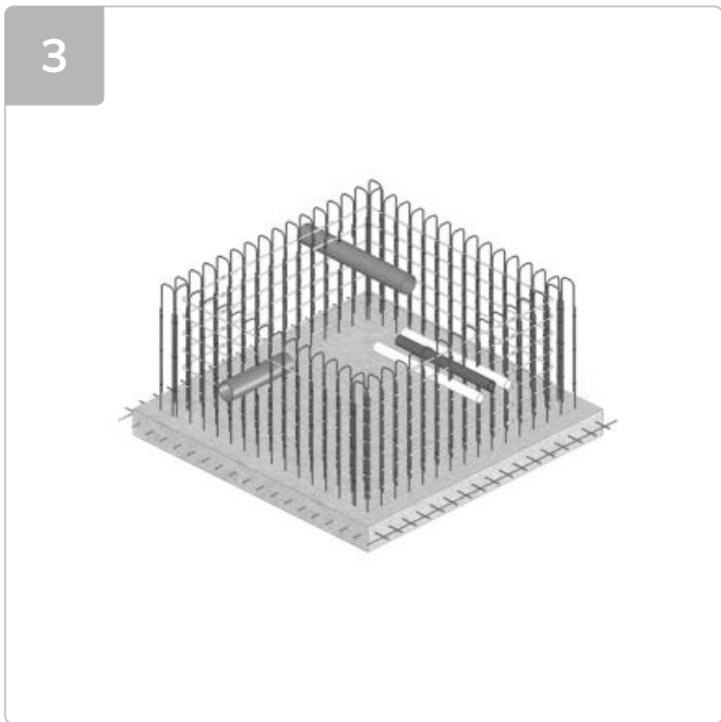
Lay inlet and discharge pipework. Allow pipework to protrude into RC box by a minimum of 100mm.
