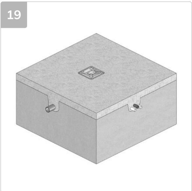
Allow concrete to cure.
