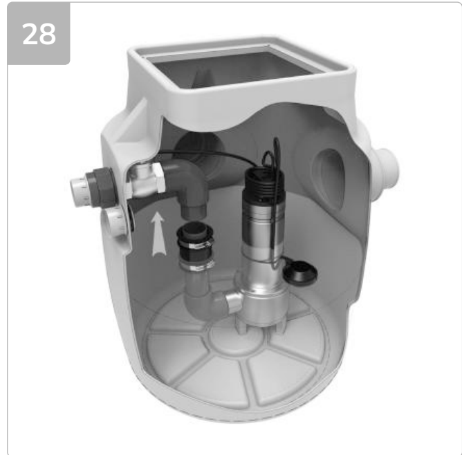
28 Slide the DC65 over the discharge arm and lower the pump in to chamber to release any trapped air. Slide the DC65 up to join the manifold to the discharge arm.
