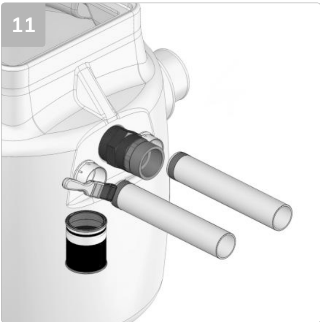
Apply high pressure glue around the first 20mm of the external face of the discharge, cable duct and vent pipe and internal side of their respective male iron.
