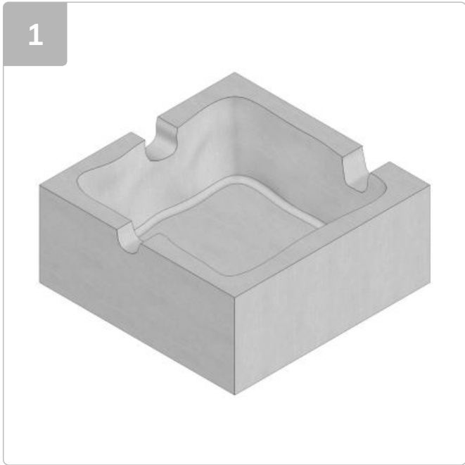
Excavate hole for chamber. Refer to section 10.0 for RC box internal dimensions.
