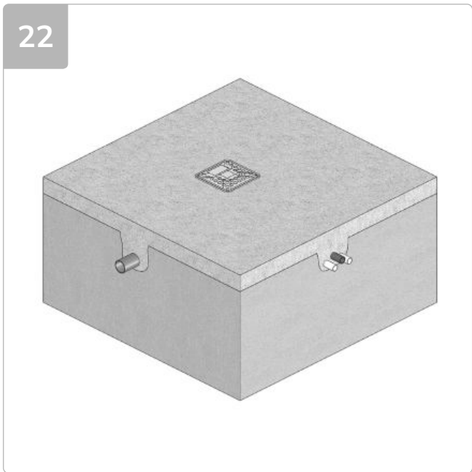
Allow concrete to cure.
