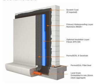
PermaSEAL 8 Geodrain is supplied in 2m wide rolls. If the foundation wall is less than 2m in height it is possible to fix PermaSEAL Geodrain horizontally with no laps. For walls over 2m fix PermaSEAL 8 Geodrain in vertical sheets with the Geotextile fabric layer facing the backfill and the black drainage layer against the wall being waterproofed.
