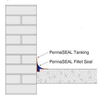
Cut a chase into the floor at the wall floor joint 20mm x 20mm deep cutting into the wall where possible. Then follow the preparation guidelines, once clean apply a coat of PermaSEAL Tanking to the area 100mm up the wall across the chase and 100mm onto the floor. Whilst still tacky apply PermaSEAL Fillet Seal to the area and chase, rounding off the fillet to create a smooth curve across the junction. Allow to dry for at least 1 hours before over coating.
