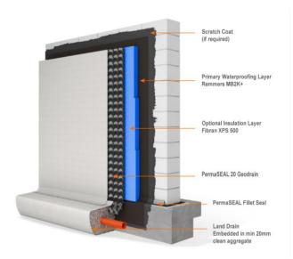
PermaSEAL 20 Geodrain is supplied in 2m wide rolls. If the foundation wall is less than 2m in height it is possible to fix PermaSEAL Geodrain horizontally with no laps. For walls over 2m fix PermaSEAL 20 Geodrain in vertical sheets with the Geotextile fabric layer facing the backfill and the black drainage layer against the wall being waterproofed.
