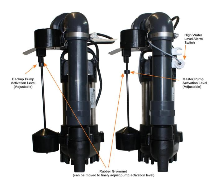
The dual pump system is designed to have one pump as the master pump and the second as a backup in case of master pump failure or a sudden water in rush above and beyond the normal volume expected.
