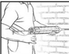
The **Ultrapoint™** works like a mastic gun. Apply steady pressure on the trigger. The mechanism is powerful and does not require a lot of force.
