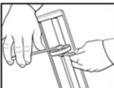
The plunger is adjustable for wear. Tightening the nuts will squeeze the rubber to tighten its fit in the barrel.
