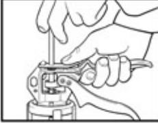
Push in the release plate at the back of the gun and pull the 'T' handle back until the plunger is out of the barrel and remove barrel. If the plunger sticks because it is dry, just pour some water into the barrel.
