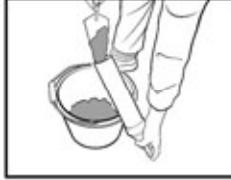
Fill the barrel and replace. Operate the trigger until the plunger makes contact with the material. The gun is now ready for use.
